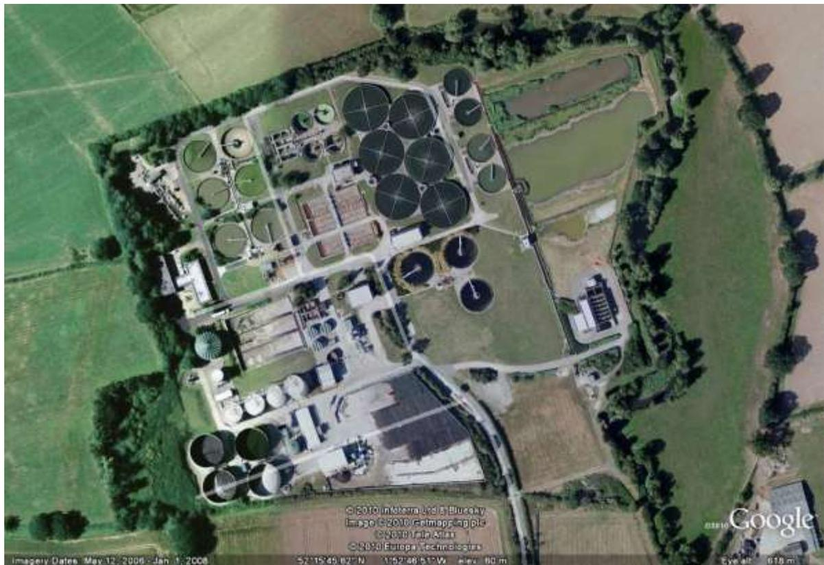
7.3.1 This is the largest STW serving Redditch Borough and uses the activated sludge process with diffused air aeration. It treats flows from the Spernal Drainage Area that serves the majority of the towns of Redditch and Studley. The Works lies outside and to the south east of Redditch Borough. Summary information for the works is shown on Table 7-2.
