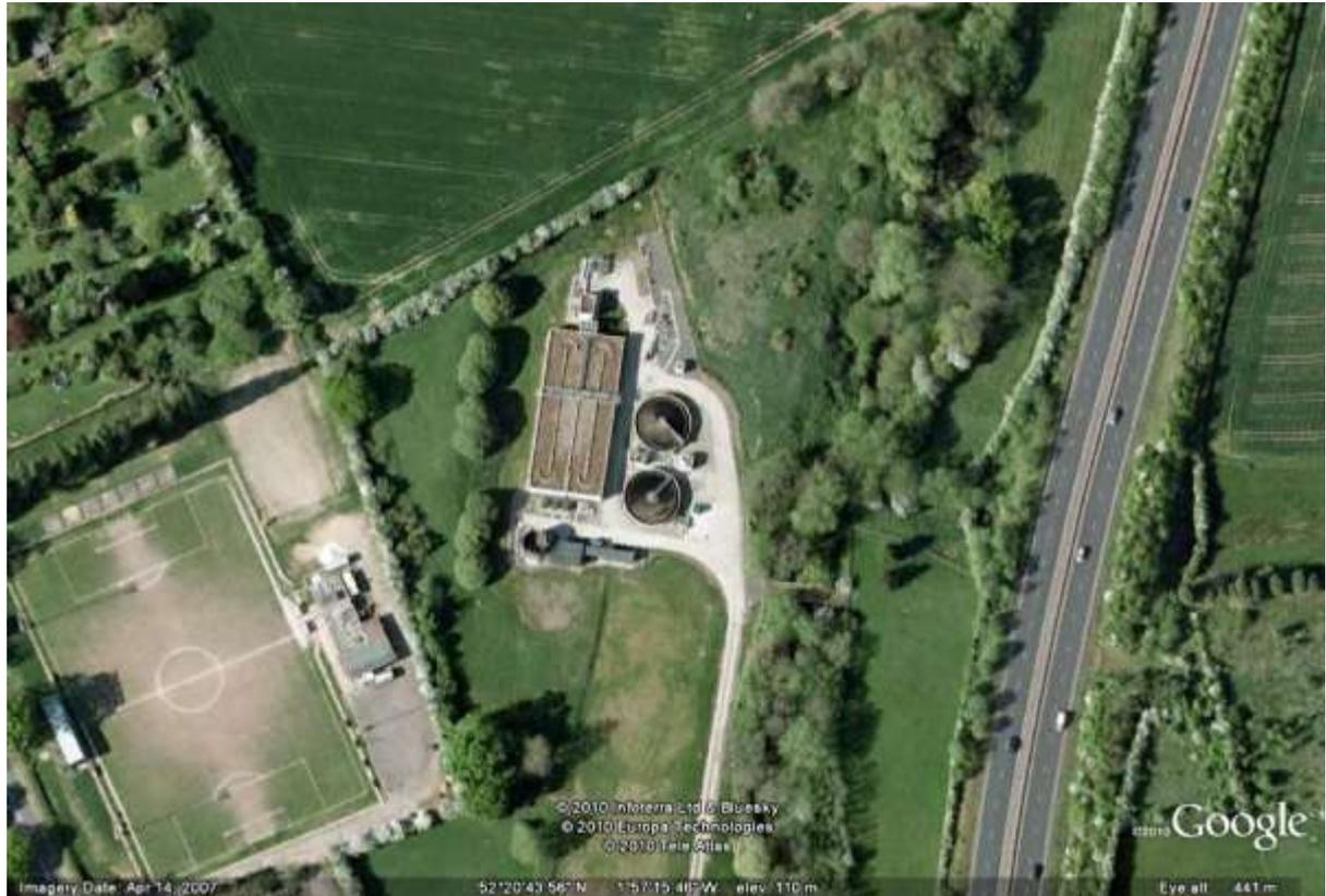
7.3.13 This STW treats flows from the Alvechurch sub-area of the Bromsgrove Rural Drainage Area in the east of the District. Treatment is provided in an oxidation ditch. Summary information for the works is shown on Table 7-5.
