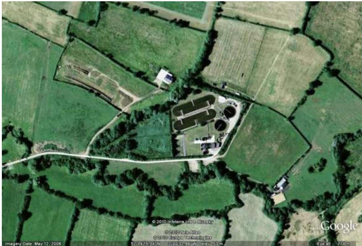
7.3.7 Priest Bridge STW is situated in the south west corner of Redditch Borough and serves the Priestbridge and Redditch Rural Drainage Areas. Treatment is provided in an oxidation ditch. Summary information for the works is shown on Table 7-3.
