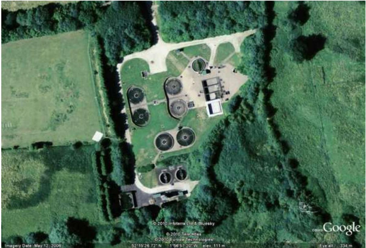
7.3.10 Astwood Bank STW treats wastewater from a small part of the Redditch Rural Drainage Area by means of re-circulating filters. It is situated on the south east boundary of Redditch Borough. Summary information for the works is shown on Table 7-4.
