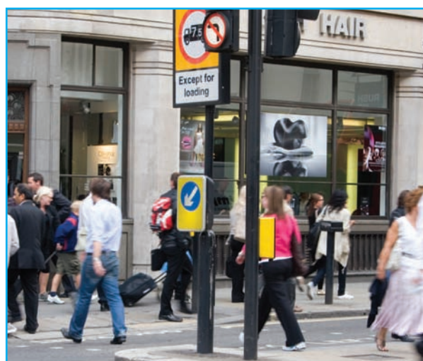
Sign to diagram 610 mounted on post. Note - yellow backing is not compulsory.
