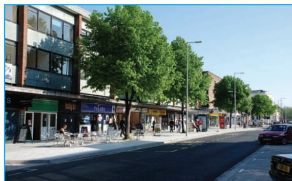
The London Road, Southampton scheme omits central line markings for part of its length.
