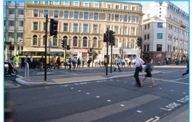
Staggered signalised crossing without guardrail
